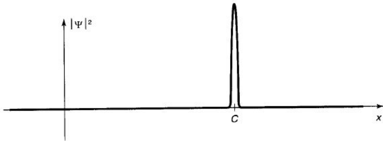
Figure 1.3: Collapse of the wave function: graph of |\Psi|^2 immediately after a measurement has found the particle at point C .
